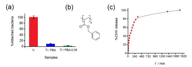
Fig. 2: (a) %Bacterial adhesion (mean ± sem) to Ti (control, 100%), Ti / poly(benzyl acrylate) PBA and Ti / PBA-0.35 after immersion in phosphate-buffered-saline (PBS) for 48 h and then in the culture medium for 2 days; (b) structure of PBA; (c) %CHX release from the Ti / PBA-0.35 coating in PBS (37 °C). Adapted from <sup>(71)</sup> and used with permission.
