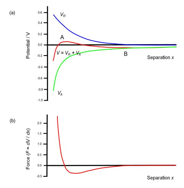
Fig. 5: Illustration of the (a) potential energy V and (b) force of attraction F between a bacterium and a plane surface as functions of separation x, as described using DLVO theory, drawn using equations (Eq. 4 – 7) with P = 1, q = 5 and S = 0.05.<sup>(56)</sup>
