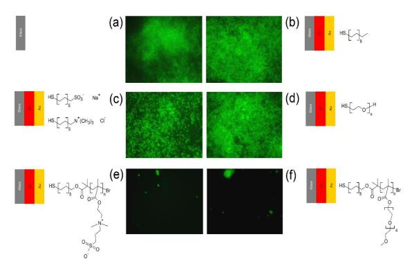
Fig. 4: Self-assembled monolayer thiol structures / polymers on Au coated glass (via a Cr adhesion layer) and resultant representative fluorescence microscopy images showing Pseudomonas aeruginosa attachment after 24 h exposure. Adapted from <sup>(122)</sup> and used with permission.
