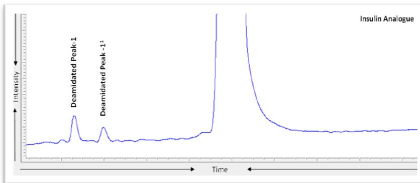
Fig. 2: IEX profile of insulin analogue showing the separation of deamidated isoforms
